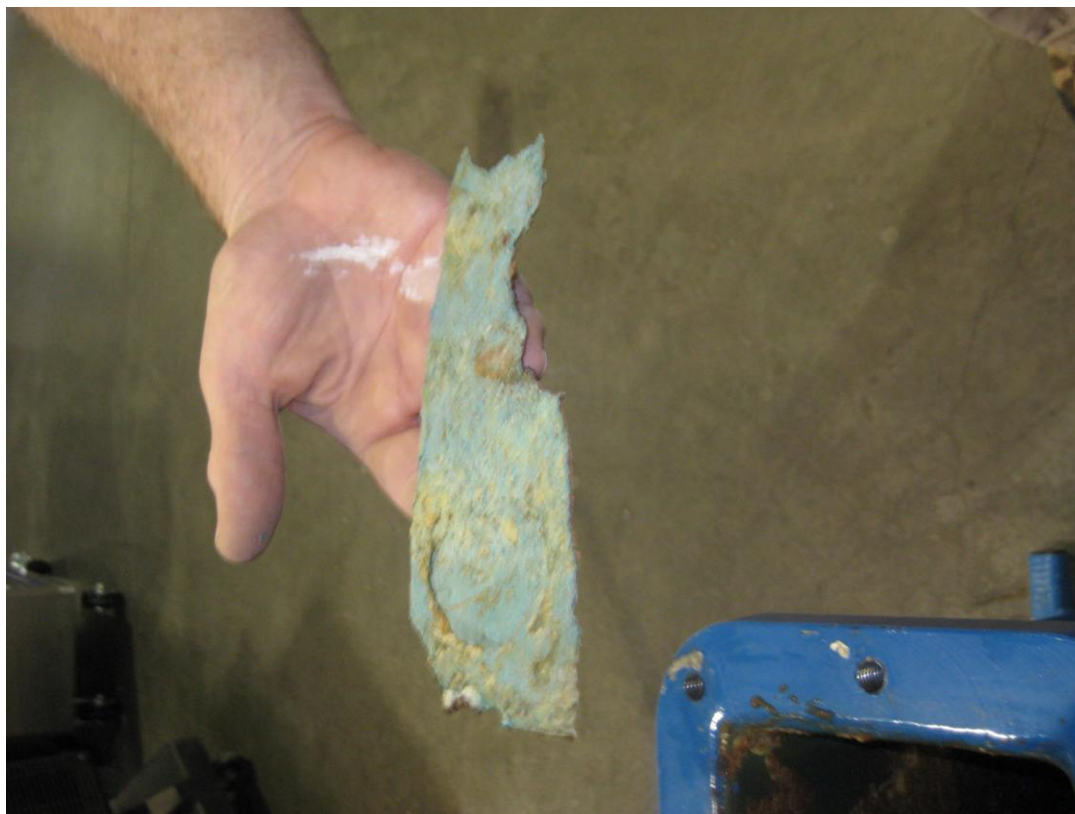
Figure 24 Piece of scale deposit from the copper electrode
