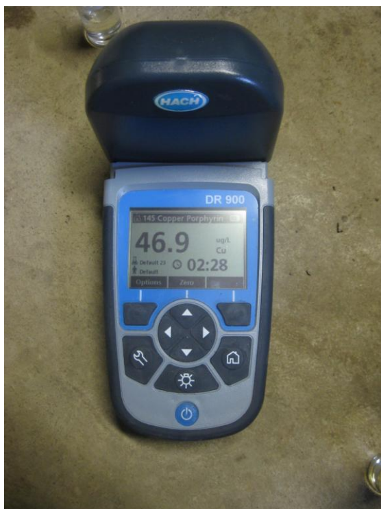
Figure 7 Hach Colorimeter used to measure copper ion concentration
